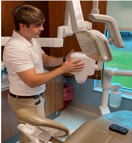
Measuring radiation from a dental x-ray unit
