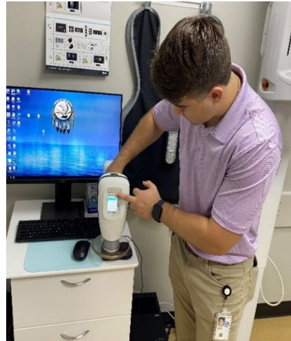
Measuring radiation from a portable dental x-ray device
