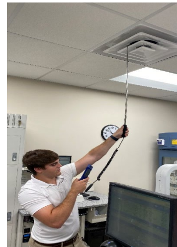
Measuring air flow in a medical clinic
